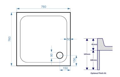
All measurement stated in mm to tolerance of +-5mm
