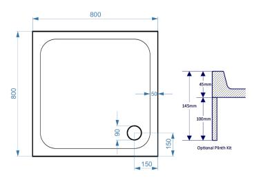
All measurement stated in mm to tolerance of +-5mm
