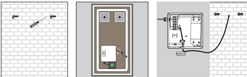
3. Unscrew the lid of the plastic box at the back of the mirror. Use the electrical connections found inside the box to connect the mirror to the main supply in accordance with the current IEE regulations. Once the connection is made, screw the lid back on the plastic box. Hang the mirror on the wall and switch on the electrical supply.
