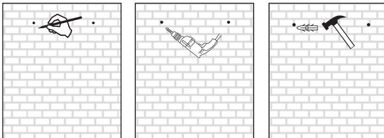
2. Drill the holes in the wall for the screw plugs supplied in the fixing kit. Ensure the holes are horizontal using a spirit level. Fasten the screws into the plugs leaving the screw head protruding about 10-8mm from the wall.
