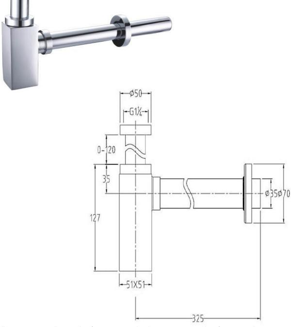
All Dimensions are in millimetres. The information contained on this page was correct at date of issue. Fitting dimensions are provided as a guide only. Some variation may occur due to manufacturing tolerances. We pursue a policy of continuing improvement in design and performance of our products and so reserve the right to change specifications without prior notice.
