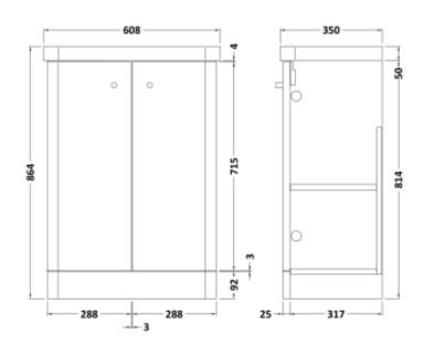
All Dimensions are in millimetres. The information contained on this page was correct at date of issue. Fitting dimensions are provided as a guide only. Some variation may occur due to manufacturing tolerances. We pursue a policy of continuing improvement in design and performance of our products and so reserve the right to change specifications without prior notice.
