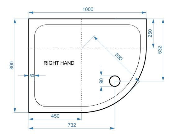
All measurement stated in mm to tolerance of +-5mm
