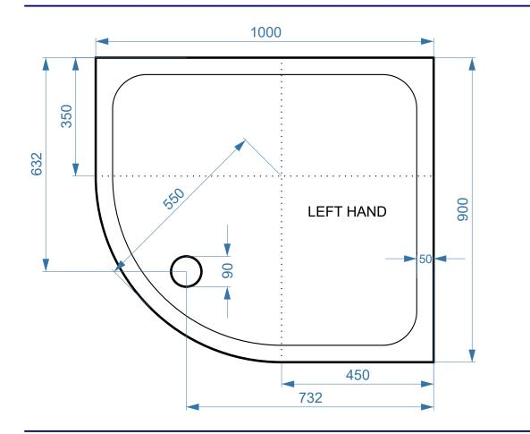
All measurement stated in mm to tolerance of +-5mm
