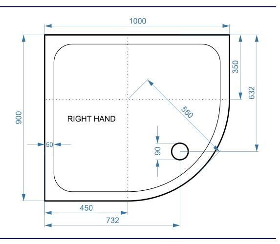
All measurement stated in mm to tolerance of +-5mm
