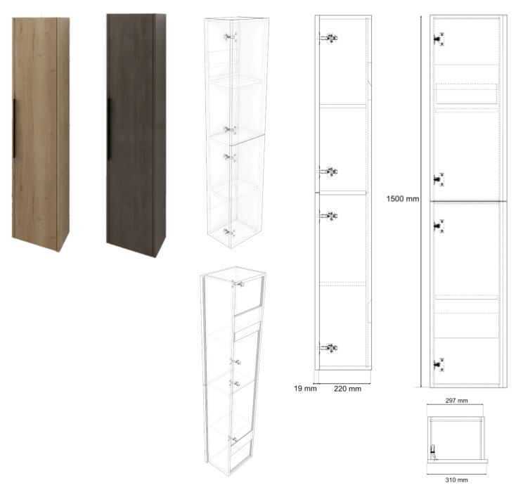
All Dimensions are in millimetres. (Drawings not to scale) The information contained on this page was correct at date of issue. Fitting dimensions are provided as a guide only. Some variation may occur due to manufacturing tolerances. We pursue a policy of continuing improvement in design and performance of our products and so reserve the right to change specifications without prior notice.
